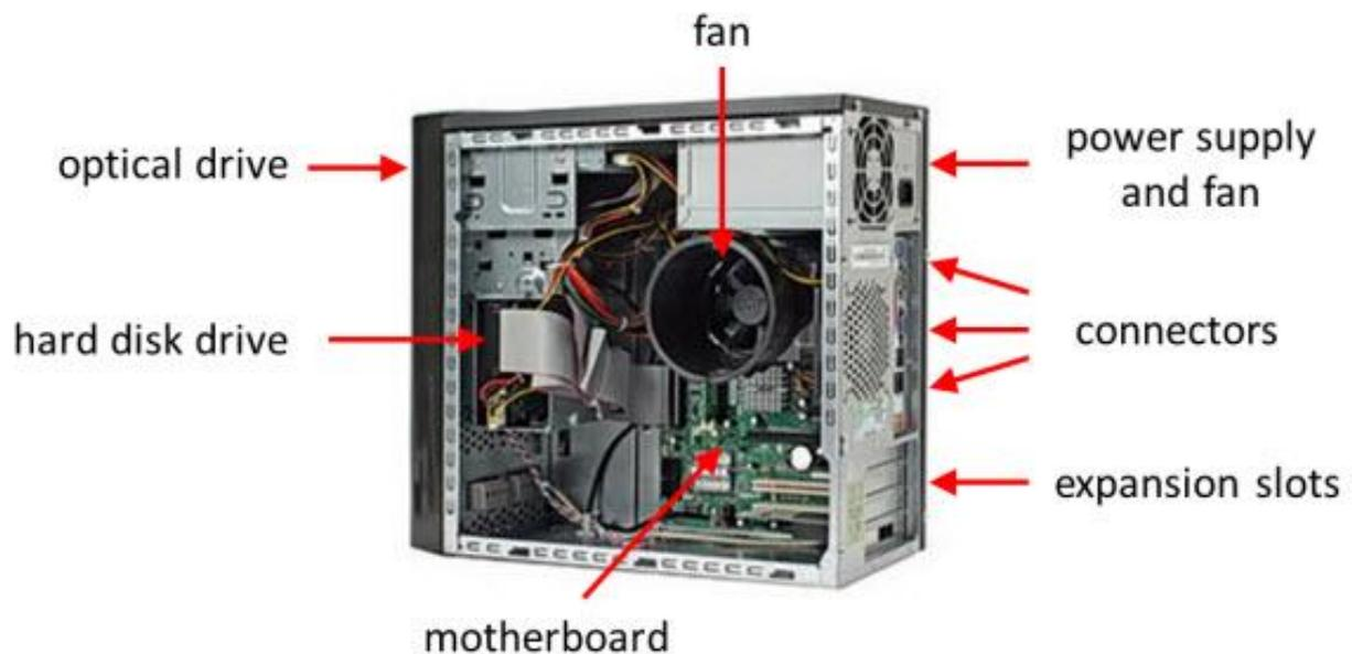
**FIG 2.2: Central Processing Unit**
